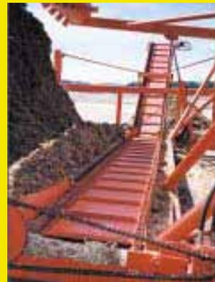
Shaft that rolls up plastic is positioned above conveyor so all remaining silage drops onto conveyor as plastic is rolled up.
