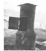
Incinerator consists of a 6-ft. dia. barrel with a 4-ft. dia. barrel mounted on top.
