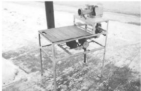
Original control lever for the wringers is used to operate the grinder.
