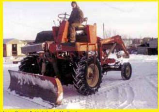
Here's a self-propelled bale hauler I built out of an old combine, a front end loader and various other components I had around the farm. It's a lot handier for hauling 5 by 6-ft. round bales weighing up to 1,000 lbs. than the tractor and dilapidated front end loader we used before.
