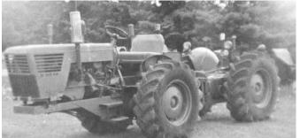
Tractor is powered by a 292 cu. in. engine out of a junked Massey 410 combine.
