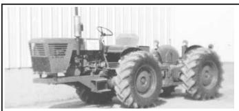
To join the rear ends, Moshondz built a hinged frame out of 3-in. angle iron.
