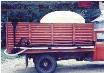
Boom is raised and lowered by a grain auger winch that's anchored to side of box.
