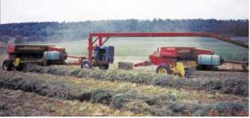
Bridge hitch goes up and over the first baler to a two-wheel engine platform ahead of second baler. A 40 hp gas engine direct-drives the rear-baler pto.
