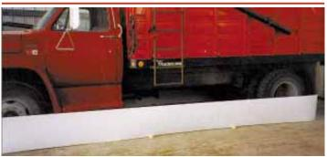
An 18-in. high wall of rigid plastic encircles each piece of equipment, keeping mice out. Eliminates the need for poisons and traps.
