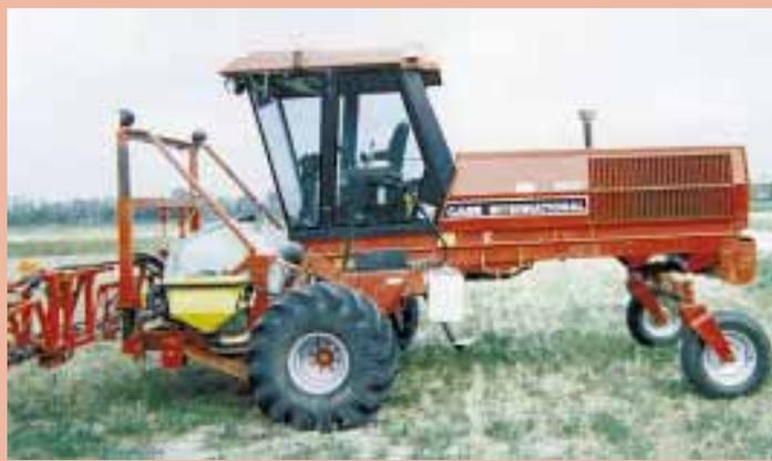
Butler built a "quick tach" 62-ft. spray boom for his new Case-IH 8830 self-propelled swather. Steel subframe supports a 300-gal. tank.
