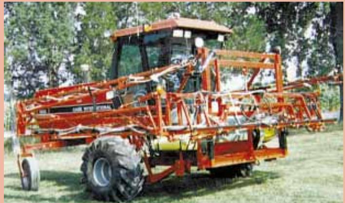
Hydraulic fold boom folds back against the sides of the swather for transport. With its
