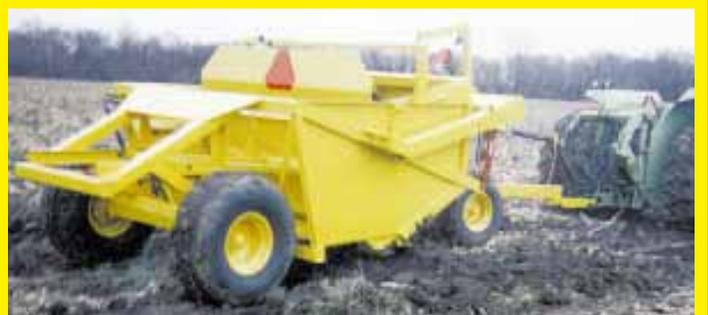
"Dirt Hog" scraper is designed to be pulled by a 4-WD or front wheel assist tractor with 140 to 250 hp. Tractor hydraulics control the unit.
