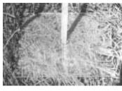
The completed meter as it's used in a field. While it was developed for a southern cool season grass/legume mix, Rayburn's calculation of 432 lbs. of dry matter per acre for each inch of pasture height is based on more northerly climes, he says.
