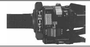
Rocker switch mounted on left handlebar operates off the ATV battery.
