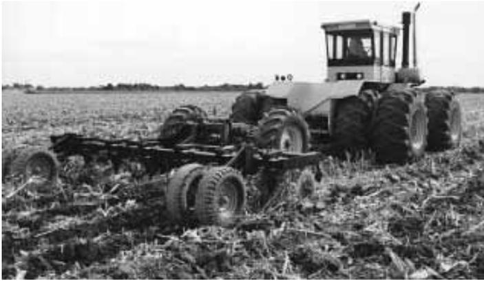
The Johnstons pull their ripper with a Steiger 4-WD, typically at a depth of 18 to 20 in.
