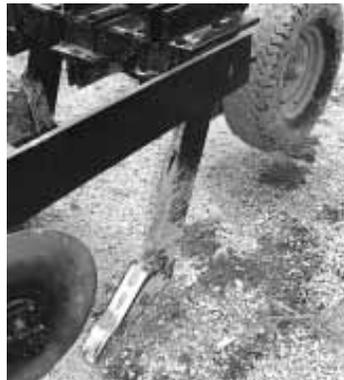
Ripper is equipped with 7 44-in. long shanks fitted with 3-in. teeth.
