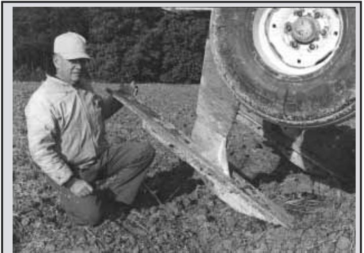
Ross Lay of Litchfield, Ill., built deep ripper he calls a "spader". It's fitted with 4-ft. blades off a road grader mounted at an angle and running 5 ft. apart. Lay runs his ripper 26 to 32 in. deep, pulling it behind a 350 hp tractor. The ripper pulls up 8-in. ribbons of claypan subsoil. Yield checks have shown a 30 bu. advantage in corn and a 6 bu. advantage in soybeans.
