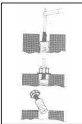
Rockmount Research & Alloys, Inc., Box 2909, Vancouver, Wash. 98668 ph 206 254-2020): "We've come up with a way to remove broken bolts and studs quickly and easily without using special equipment. The stud extraction procedure requires our Brutus electrode, a nut, and a washer. The Brutus electrode has a non-conductive coating that eliminates side arcing. It can be used on tool steel, stainless steel and hardend steel.
