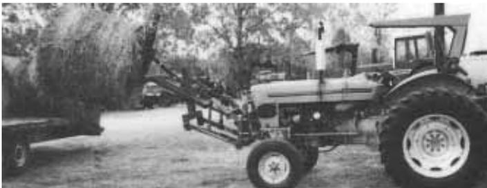
Front bale mover uses an extension designed for a rear-mount 3-pt. A heavy-duty frame that supports the bale spear.
