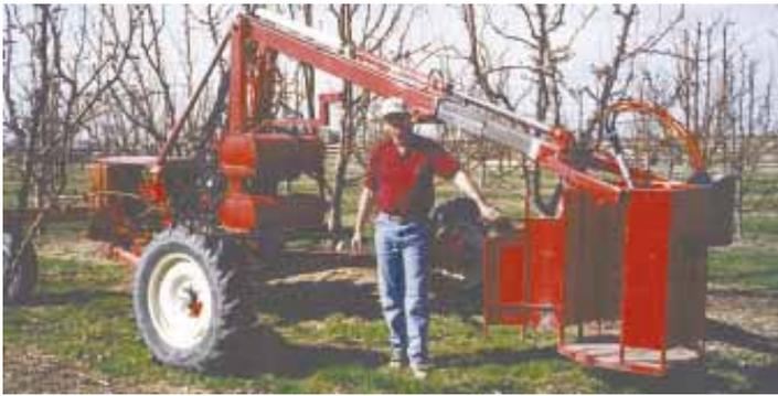
Hydrostatic drive, self-propelled tree pruner is equipped with a telescoping boom that rotates 180 degrees, and a self-leveling basket.
