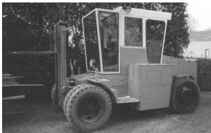
**Roesner built his bi-directional forklift around the chassis of a 1961 Ford F-700 truck.**
