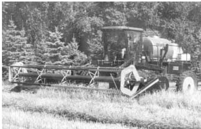
**A 25-ft. MacDon swather header mounts on front of the Walker 44, providing another use for the expensive self-propelled rig.**
