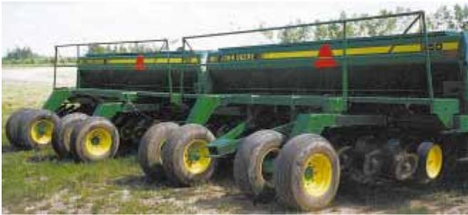
For extra flotation he added hubs and spindles on back of drills and fitted them with the original wheels and tires from the front.
