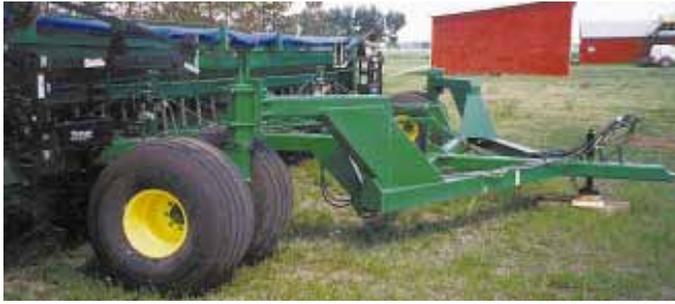
Manning built a new beefed-up hitch for drills and mounted a pair of big dual castor wheels on it.
