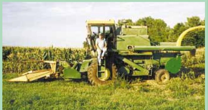
Stoll equipped his Deere 4420 combine with parts from a Deere pull-type forage harvester, mounting the harvester's header on front and the auger and blower on back. Lets him shell corn conventionally and chop silage into a wagon at the same time.
