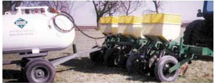
Fertilizer boxes were moved to rear of planter toolbar. Deere plow coulters mount ahead of each anhydrous shank.
