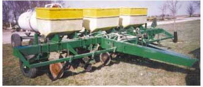
Kirk used a 6-row Deere planter toolbar and Deere dry fertilizer attachment to build rig. Lets him apply dry fertilizer and anhydrous ammonia at same time.
