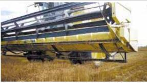
"Recutter" mounts underneath and behind Mosby's 30-ft. New Holland 971 header.
