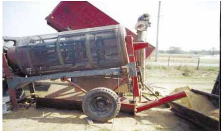
Two-stage auger system automatically dumps screenings into a big tractor bucket.
