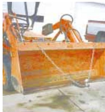
Ball hitch lets bucket push trailers. Chains can be used to support hitch.
