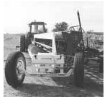
Hydraulic-lift trailers are equipped with a ramp on one side, allowing you to back drill over ramp and lock it down.
