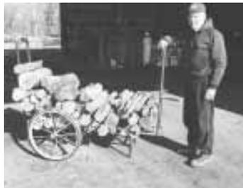
He uses this two-wheel cart to haul wood. He built a 6-ft. long by 3-ft. wide two-wheel cart. The frame is built out of scrap pipe and fitted with wheels off a junked weed mower.
