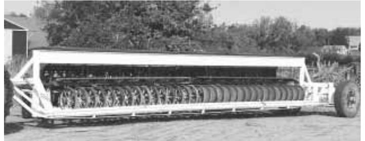
International 150 32-ft. hoe drill is shown mounted on 2-wheeled, 41-ft. long trailer.
