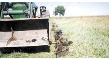
I built a nifty fence-line digger to keep weeds from grounding out an electric fence around a pasture. It consists of a 10-in. long Deere tractor cultivator shank and a 12-in. dia. Deere disk hiller blade.
