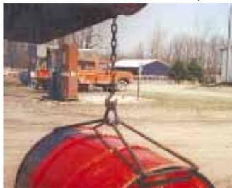
the lip of the barrel. The triangular hooks are joined by a ring that allows me to lift 55-gal. barrels of oil with my tractor loader to set in my shop. (Fred Lewis, 12740 Ridge Hwy., Britton, Mich. 49229; ph 313 439-2164)
