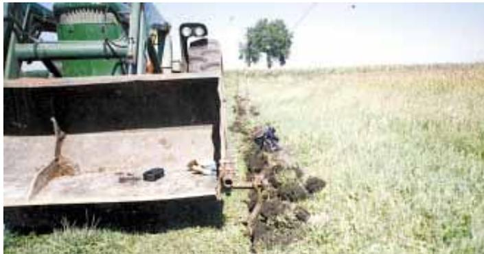
I built a nifty fence-line digger to keep weeds from grounding out an electric fence around a pasture. It consists of a 10-in. long Deere tractor cultivator shank and a 12-in. dia. Deere disk hiller blade.
