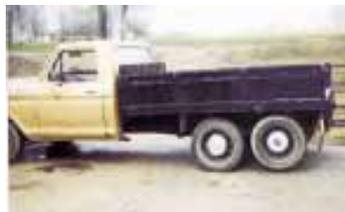
ride about 2 in. off the ground. When the pickup's loaded heavy, the wheels drop to the ground. Most of the parts for the project came out of my scrap iron pile. (Billy R. Hatfield, 3409 Hwy. 63, Speedwell, Tenn. 37870; ph 423 869-8311)
