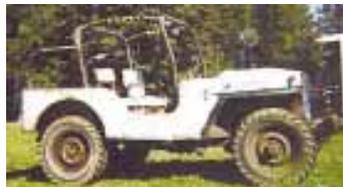
a Buick car and fitted with a roll bar for use as a "dune buggy". I reassembled the Jeep and installed a power steering unit and steering column out of an old GM car. It has all the power, speed and traction I need, and has even pulled tractors and trucks out of the mud.
