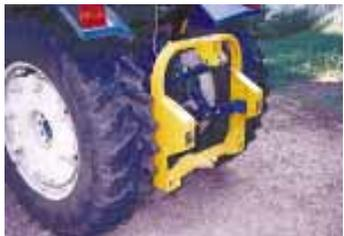
an automatic latch on bottom so the operator can hook and unhook implements from the tractor seat. No jack is needed and the design keeps the hitch stable.
