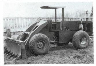
He borrowed the 16 by 16 tires from a Cockshutt 428 self-propelled combine. The tractor has five hydraulic cylinders two 48 by 4 in. cylinders to lift the loader arms, two 20 by 4-in. cylinders to lift the
