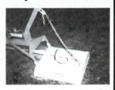
A universal joint at the hinge of the mower deck allows the deck to pivot up and down while mowing.
