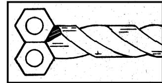
angle so the drill will run true. Klaus recently pointed out in an article in Woodshop News that you can vary the angle slightly to 120 degrees by using two standard machine nuts as a guide. Just grind the tip down to fit the angle of the two nuts and it'll work fine, he notes.
