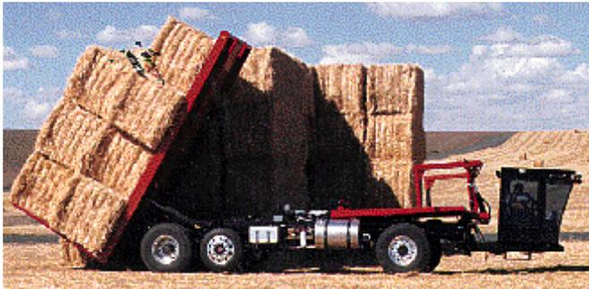
Loading table raises vertically to stack two bales on top of each other on the loading deck. Machine can load and stack 800 1-ton bales per day under ideal conditions.
