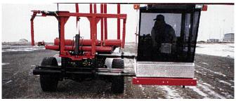
Telescoping cab moves off to the side when loading bales and then shifts back in front for road transport.
