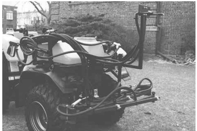
Kit includes 25-gal. tank, bracket, and two boomless nozzles that mount on ATV. (Note: 12-ft. boom on ATV shown above was used by a chemical company for test plot work.)
