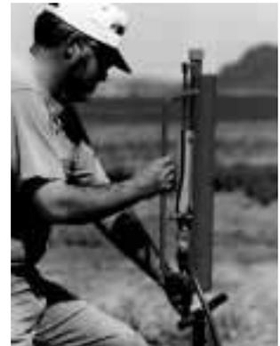
An inner sleeve clamps in place. Air pressure lifts the device off the sleeve, then drives it downward at a rate of 80 to 85 strokes per minute.
