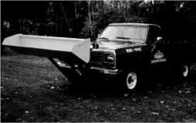
Bucket mounts on standard Fisher snowplow lift arms and uses existing hydraulic cylinders. It can be raised 3 to 4 ft. off the ground.
