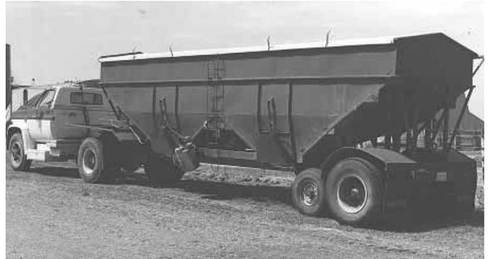
Trailer has divided hoppers which allow Henry to haul 350 bu. of wheat seed in one and 10 tons of dry fertilizer in the other. He can haul 670 bu. of grain legally.
