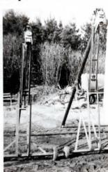
augers, the frame can be moved forward or backward. Both augers are driven by electric motors mounted on top.'
