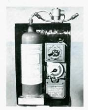
Compact Accudose unit treats up to 65,000 cu. ft. of enclosed area per treatment. One dial controls frequency of treatment, the other regulates dosage.
